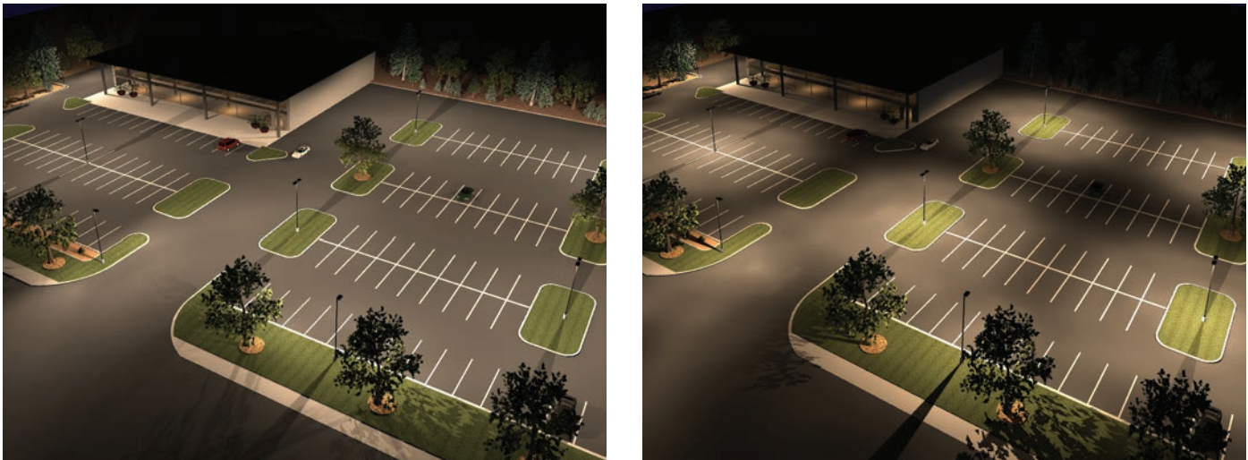
Prevail A40 LED 14 Fixtures = 2,002 Total watts
