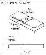
Photocontrol cover is precision machined from corrosion-resistant 6061-T6 aluminum and is secured to bollard head with tamper resistant stainless steel hardware. The photocontrol option is available in dedicated 120V or 208-277V. When specifying a photocontrol option make sure to designate the appropriate voltage within the catalog logic.
