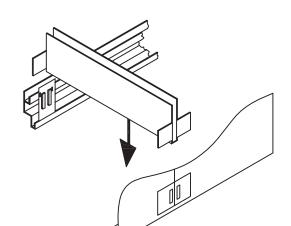
STEP 6 PROVIDE BLOCKING (NOT BY NEO-RAY) WALL INSTALL SHIELDING ELEMENT.
