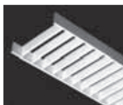
S62 Lateral Louver 3/16" high x 3/4" o.c., aluminum lateral louver white finish.
