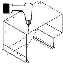
Using gusset as a guide, drill holes for & mount gusset in aluminum filler. Screw in all aligning clips. Remove and keep spacer blades.
