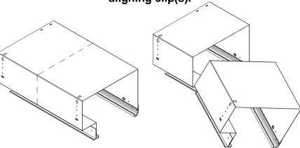
Measure the distance between the last steel housing & the desired end of run. Cut aluminum housing to fill remaining space.
