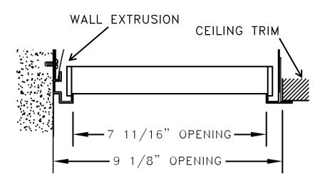
Cut ceiling to interface with fixture as shown. Level with indicated face of ceiling rail.
