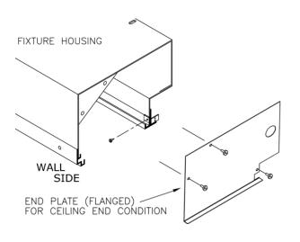
If the end of the first fixture abuts a wall, attach the supplied end closure to the wall in-line with the fixture, as shown.
