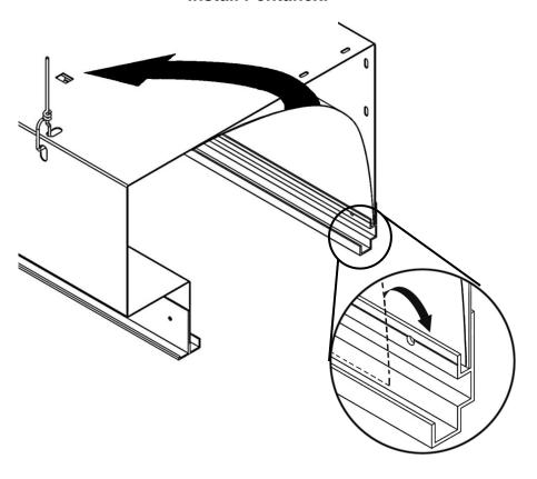
Push the left edge of the Pentaflex firmly against the end of the run, carefully tucking the top edge into the leftmost lance on the housing. Continue in a like fashion to the center of the run.
