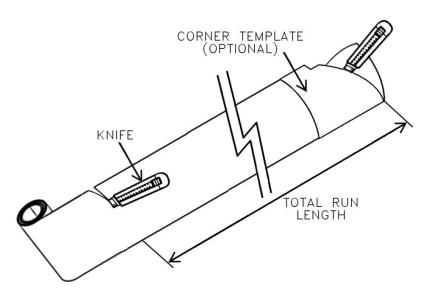
Using a sharp knife, cut strips from the roll of Pentaflex (shipped separately) to fit the full length of the run, flush with the ends of the wall rails. (If more than one strip is needed, leave a 3-4" overlap in the center.) If there is a corner at either end of the run, use the supplied Pentaflex corner template to cut the corner's profile at the proper end of the strip.
