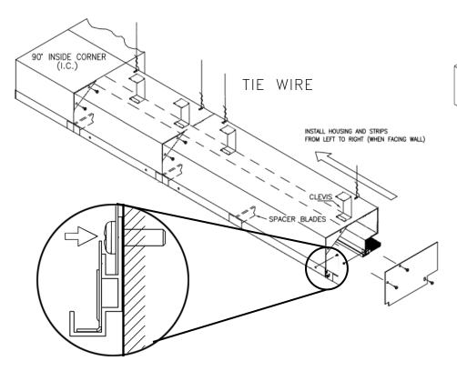
Determine proper placement of fixtures using submittal drawing. (Lighting should be centered along wall.) Working from left to right, mount each fixture to the wall & to all previous fixtures as shown, with screws. Attach & configure all necessary wiring, including feeds, as needed. Attach supporting tie wires to the holes in the rear of each fixture, as shown.
