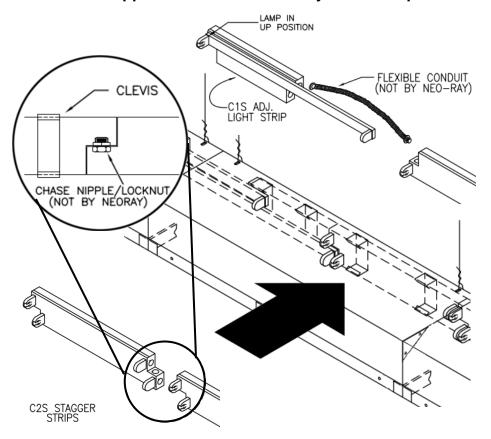
Working from left to right, remove the cover of each light strip & snap them into clevises, joining adjacent strips with chase nipples and lock nuts, and wiring them to the previous light strips in the run. At the end of the run, mount the adjustable light strip as shown, and extend to desired length.
