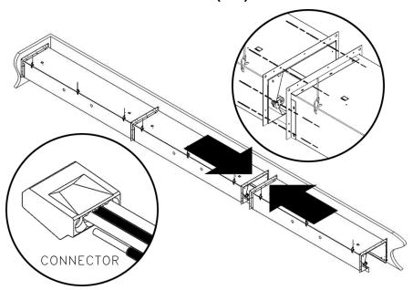
Attach each intermediate (INT) fixture to the run, using screws & nuts to pull flanges together. Connect appropriate wiring where desired using supplied electrical connectors.
