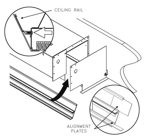
Extrusions are supplied in twelve-foot lengths (to minimize seams). Attach the ceiling extrusions to each fixture as shown & both end plates. Insert alignment plates between segments, making sure each is flush & level.
