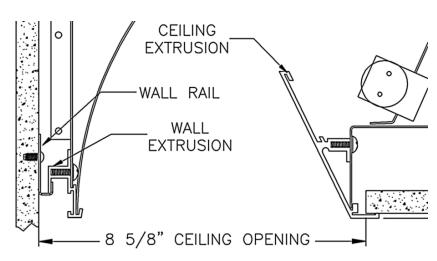
Cut ceiling to interface with fixture as shown. Level with indicated face of ceiling rail. Check to make sure all parts are properly seated & flush.
