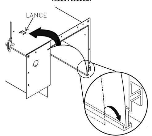
Push the left edge of the Pentaflex firmly against the end of the run, carefully tucking the top edge into the leftmost lance on the BOR housing. Continue in a like fashion to the center of the run.
