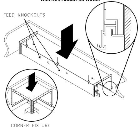
Determine proper placement of fixtures using submittal drawing. (Lighting should be centered along wall.) Check that the wall rail channel is clear of debris. If there is a corner fixture to the left of the BOR, mount it first. Attach & configure all necessary wiring, including feeds, as needed. Hang the fixture over the wall rail channel and attach supporting tie wires to the holes in the rear of the fixture, as shown.
