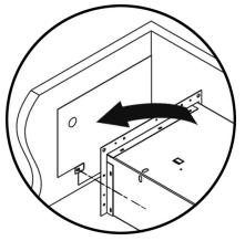
If the end of the BOR abuts a wall, attach the supplied end closure to the wall in-line with the fixture, as shown.
