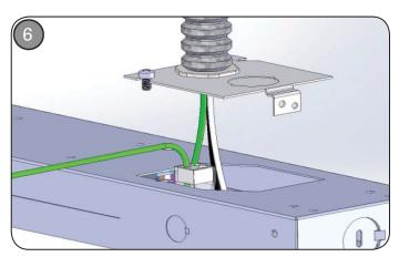
Bring power to remote enclosure. Remove access plate, make appropriate wire connections and re-secure access plate to remote enclosure.
