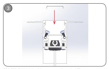
FOR FSR ONLY: Using (2) 8-32 screws from the LED pan assembly, install aperture guide snugly to ensure housing opening does not open or close during installation.
