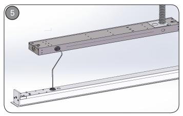
Each fixture length, Individual or Continuous, is supplied with a pre-wired remote driver enclosure. Enclosure can be dis-connected; ensure to mark enclosure and fixture if dis-connected. Remote enclosure is supplied with MAXIMUM length low voltage, plenum rated cable. Cable can be shortened if desired. DO NOT lengthen cable.
