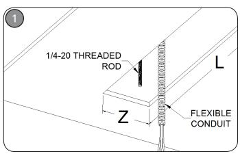
Install shielded cable to accommodate electrical feed point. Install 1/4-20 tie rods in specified locations as shown on factory submittal drawings. Cut hole in gypsum board (or other substrate) as specified on factory submittal drawing (dimensions "Z" & "L"). NOTE: FSR requires bracing around opening to secure flange.
