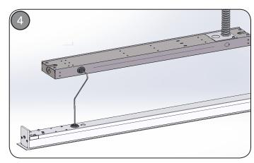
Locate remote driver in an accessible location. Either an access panel or other accessible location may be needed to service driver after final installation.
