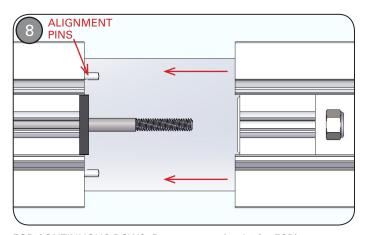
FOR CONTINUOUS ROWS: Repeat step 2 (and 3 for FSR) to prepare fixture. Slide fixtures together ensuring alignment pins are in the correct position. FOR CONTINUOUS RUNS: Insert #8-32 bolt through both fixtures. Using a 9/64" allen wrench and a 11/32" nut driver draw fixture housings together. Repeat until to complete entire fixture run.
