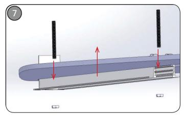
Draw fixture tight to ceiling using 1/4-20 tie rods through the appropriate knockouts on fixture housing. Secure with nuts until flange is snug. Refer to next page for detail. NOTE: FSR must be secured with tie-rod.
