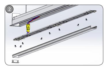
Prior to installing fixture, remove lens, top access plate, and diffuser bracket. Turn fixture over. Remove screws and carefully lift LED pan assembly from housing frame, disconnect low voltage connection and store pan assembly in a safe place.
