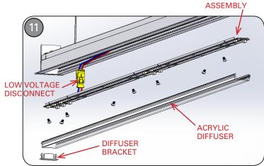
With fixture securely secured in opening, reconnect the low voltage disconnect from the driver to the LED pan assembly. Carefully tuck all wiring back into fixture. Reinstall screws to secure pan assembly back into housing. Reinstall acrylic diffuser and then diffuser bracket in fixture housing.
