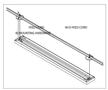
STEP 10: ALIGN FIXTURE TO HAVE IT STRAIGHT AND LEVEL BY ADJUSTING AIRCRAFT CABLE.
