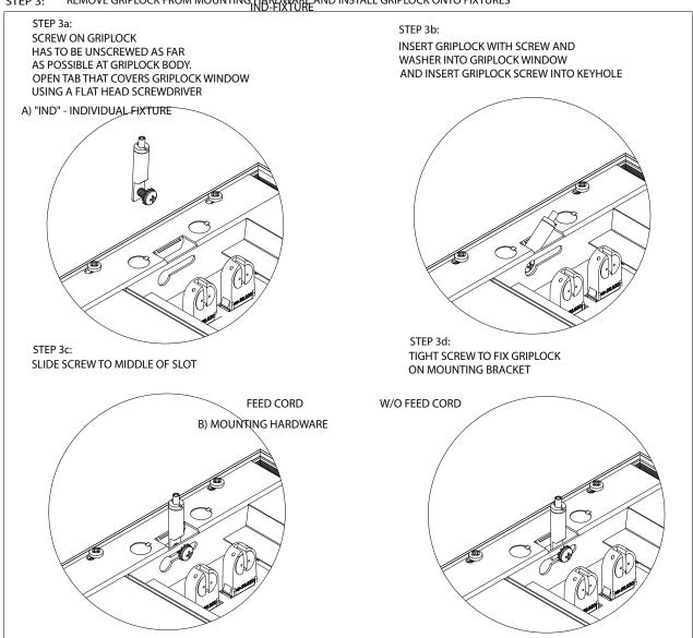
NOTE: INSTALL GRIPLOCKS AT BOTH ENDS OF IND FIXTURE
