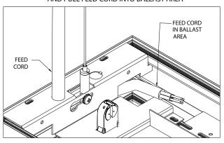
STEP 6: MAKE ELECTRICAL WIRE CONNECTION AT FEED
