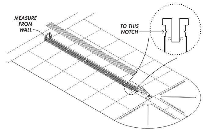
Next install a small piece of cap to cover the wireway on the other side:
