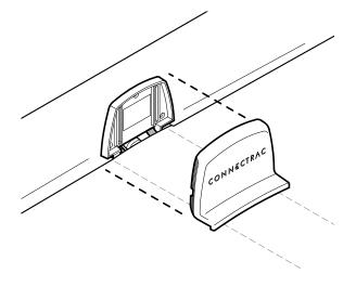
After the carpet is installed, the frontplate can snap onto the backplate.
