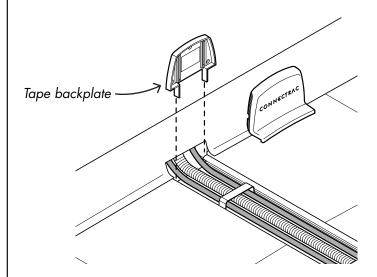
First use mounting tape to stick the backplate against the wall base, making sure to align the legs in the aluminum bottom track
