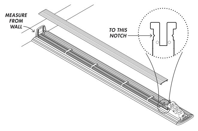
Next install a small piece of cap to cover the wireway on the other side:
