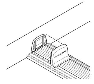
The frontplate can snap onto the backplate after the top cap is installed in the next step.
