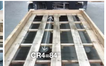
FIG. 5 – CRATE OR A-FRAME – CROSS RUNNERS Underside view with 84" forks
