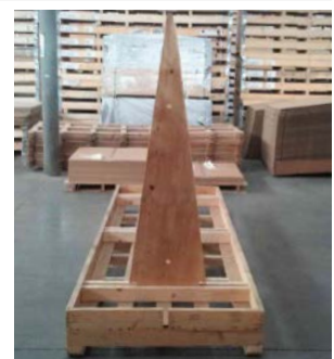
FIG. 2 A FRAME LAM-CRATE 124 x 44 / LAM-CRATE 144 x 33 = 40 pcs max capacity 3+ and 20 pcs max capacity 5.6
