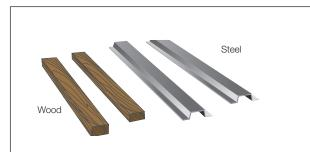
1. For wall or ceiling application, Solo can be installed using wood blocking or steel furring channels. Install wood blocking or steel furring (hat) channel at 610mm (24") on center.
