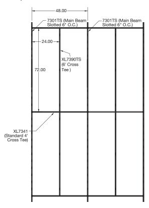
2.3 For 2' x 8' panels: Prelude XL HD main beams that are pre-slotted 6" O.C. (item 7301TS) for Torsion Spring panels are installed every 24" O.C. Then 24" Prelude cross tees (item XL7328) shall intersect the main beams at 90 degrees every 96". Springs on the panel will be inserted into main beams only.
