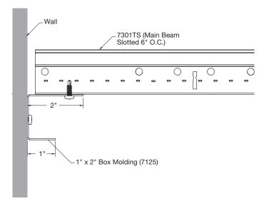
**2.7** Cut edges are held down against the molding by inserting a 7126 Spreader Hold Down into the molding, between the upper and lower flanges, over each cut panel. The 7126 Spreader Hold Down is 10.625" long, so use the appropriate amount of hold downs for the panel edge dimension.
