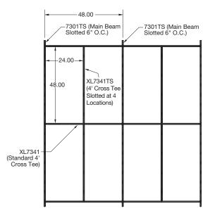
**2.2** For 2' x 6' panels: Prelude XL HD main beams that are pre-slotted 6" O.C. (item 7301TS) for Torsion Spring panels are installed every 48" O.C. Then 48" Prelude cross tees (item XL7341) shall intersect the main beams at 90 degrees every 72". Then a 72" Prelude cross tee that is slotted (item XL7390TS) at three locations shall be bridged in at the center of the 48" cross tees to run parallel with the main beams. Springs on the panel will be inserted into main beams and cross tees.
