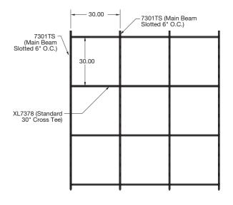
Hangers and bracing are to comply with all local code requirements. The suspension system shall be properly installed and leveled using not less than 12 gauge galvanized steel wire. Suspension system installation shall conform to ASTM C636 requirements. The suspension system for all panel sizes must be leveled to within 1/4" in 10' and must be square to within 1/16" in 2'. 90° Alignment Clips (item 7134) can be used to assure the grid system meets the squareness requirement.
