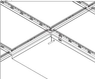
The Suction Panel Removal Tool (item 7130) is for unperforated panels only. Place the device on the corner edge of the panel and gently pull down until the spring is accessible. Push the spring together and pull down gently to release the panel from the main beam.
