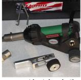
Note: Should another type of welding robot be used, such as Leister robot, care must be taken in the choice of tip as for most cases the opening of the tip is more than 2mm. This could damage the flooring and lead to a seam failure.
