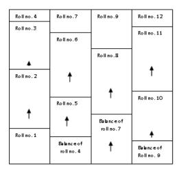
G. Roll material is stretched slightly when it is rolled at the factory. At the job site, the installer should allow all rolls to relax for a minimum of two hours before gluing or cutting material.
