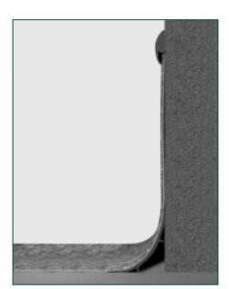
Figure 8 CS capping strip
