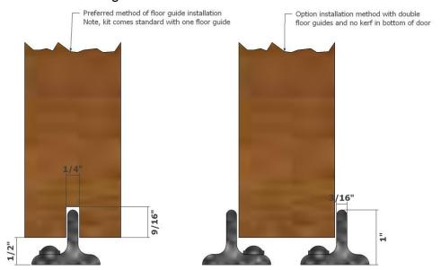
If you want the alternative option shown in picture with double guides, be sure to order an extra floor guide. Otherwise cut a 1/4" wide kerf centered in bottom of door. To determine depth of kerf cut, subtract desired gap under door from 1" and add 1/16", so for a ½" gap under door you would have a 1/4" wide and 9/16" deep slot/ kerf. This is easiest to do with a router and a slot cutter.
