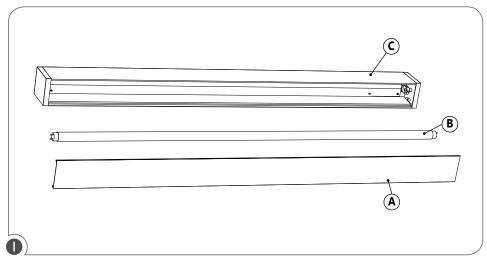
**NOTE:** Before attempting to verify and replace the ballast, ensure that the power to the fixture's circuit is turned off. Remove optics (A) and lamps (B) from the fixture (C).
