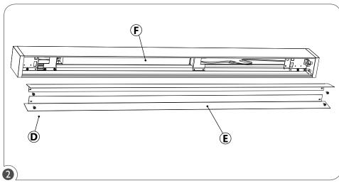
Remove reflectors retaining screws (D) and remove reflectors (E) to reveal the ballast (F).
