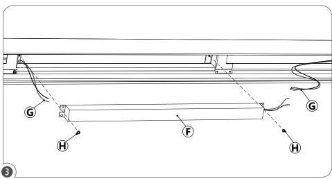
Disconnect wires from the ballast (F) using the quick-wire connectors (G). Remove the ballast (F) retaining nuts (H).
