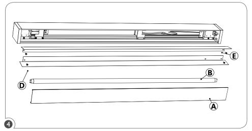
Put the reflectors (E) back in place and fasten retaining screws (D). Re-install the lamps (B) and optics (A).
