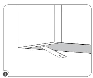
Using the provided tool. Starting at one end of the fixture, insert the bent end of the tool into the fixture lens as shown in the above illustration.
