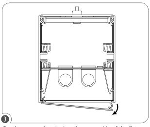
Continue removing the lens from one side of the fixture.
