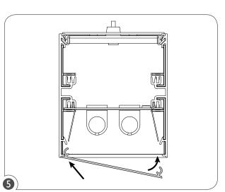
To install, slide lens inside the fixture by starting with one side and push inwards into the fixture until the lens snaps in place.
