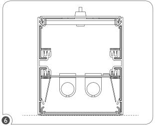
Make sure that the lens is firmly seated and leveled along the whole lenght of the fixture.
