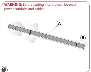
Ensure that the power to the fixture's circuit is turned off. Cut hole (A) in drywall and place 1/4-20 threaded rods (B) according to the dimensions on the shop drawings. Tape and finish around the edges.
