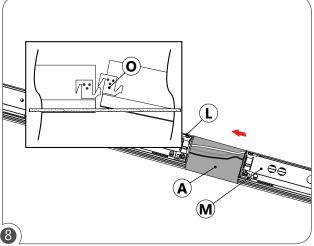
Insert the second sections (M) into the drywall hole (A). Slide the sections together and hook the joining hooks (O) to each other to join sections and aligning ½-20 threaded rods with the mounting holes.
