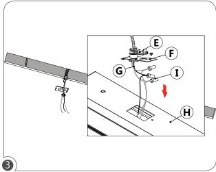
Install BX cable connector (E) through the power plate (F). Wire BX cable wires (G) to fixture (H) using the wire nuts (I). Push connected wires into fixture (H). Fasten knockout plate (F) to fixture (H).
