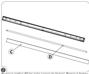
Remove optics (C) to gain access to lamps. Remove lamps (D) if installed.
