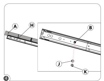
Push fixture (H) into cut hole (A) in drywall, aligning \( \frac{1}{4} - 20 \) threaded rods (B) with the mounting holes on top of fixture (H). Secure fixture (H) with washers (J) and nuts (K).
