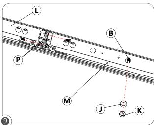
Secure the second section (M) to the  $\frac{1}{4}$ -20 threaded rods (B) with washers (J) and nuts (K). Secure joinning brackets (P) to each other using the supplied screws.
