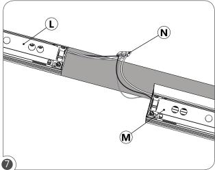
Make wire connections with quick-wire connectors (N) between the joining sections (L) and (M).
