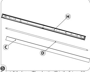
Re-install the lamps (D) and optics (C) in the fixtures (H). Power can now be turned on.
