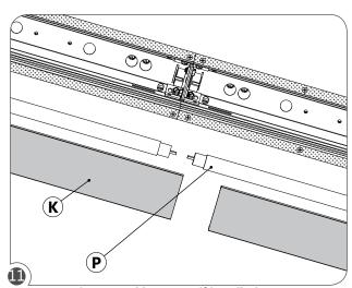
Remove optics (K) and lamps (P) if installed.
