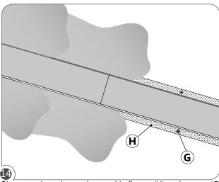
Plaster and sand over the spackle flange (H) and screws (G) of both sections to create a smooth finish.
