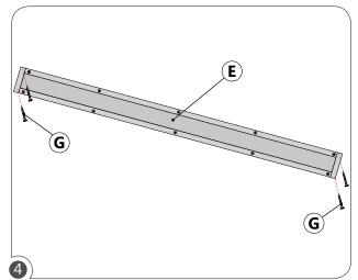
Check the fit of the fixture (E). If the fixture (E) appears bowed or too loose, remove screws (G) on one side of the fixture (E), adjust the fixture (E) so that it fits flat and snug, and reinstall screws (G). (Ensure fit of the lens by removing and reinstalling before plaster)
