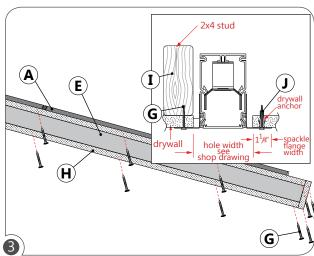
Align fixture to the pre-cut drywall opening (A) and insert fixture (E). Fasten fixture (E) to the drywall by drilling screws (G) through the spackle flange (H). Wood blocking (I) or drywall anchors (J) must be used to reinforce the screws (G) to the drywall.
