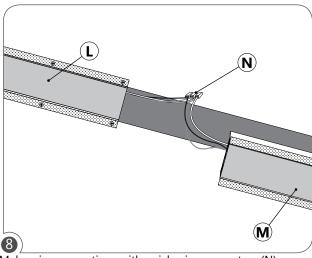
Make wire connections with quick-wire connectors (N) between the joining sections (L) and (M).
