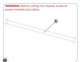
Ensure that the power to the fixture's circuit is turned off. Make an opening (A) in drywall according to the dimensions on the shop drawings.
