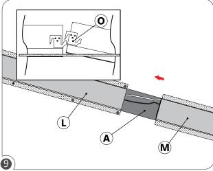
Insert the second section (M) into the drywall hole (A). Slide the sections together and hook the joinning hooks (O) to each other to join sections.
