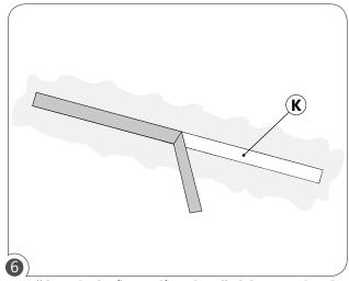
Install lamp in the fixture (if not installed) by removing the optics (K) and placing it back carefully. Remove blue tape from optics (K) **BEFORE** the last plaster layer is fully dry. Power can now be turned on.
