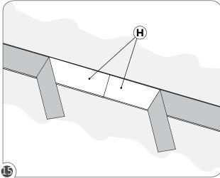
Follow steps **1** to **4** for the next sections. Remove blue tape from optics (K) **BEFORE** the last plaster layer is fully dry. Power can now be turned on.
