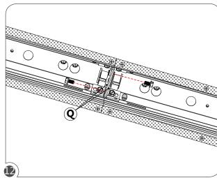
Secure joinning brackets (Q) to each other using the provided screws.
