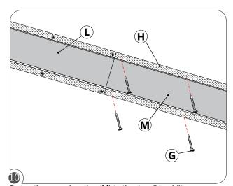
Fasten the second section (M) to the dywall by drilling screws (G) through the spackle flange (H). Check the fit of the second section (M). If the section (M) appears bowed or too loose, remove screws (G) on one side of the section (M), adjust the section (M) so that it fits flat and snug, and reinstall screws (G).
