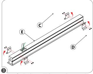
Rotate safety brackets (D) 90 degrees. Using screws (C) from step 2 place safety brackets (D) back to the fixture (E) using top row of holes (for screw slot and tegular T-bars, the safety bracket (D) needs to be fastened with the bottom row of holes).
