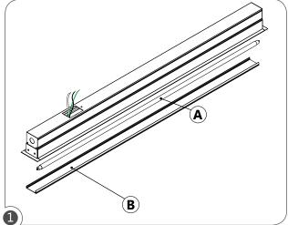
Ensure that the power to the fixture's circuit is turned off. Remove optics (A) and lamp (B) if installed
