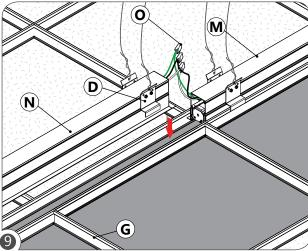
Make wire connections with quick-wire connectors (O) between the joining sections (M) and (N). Lower the second section (N) onto the T-bar runner (G). Ensure that the safety brackets (D) sit above the T-bars (G).
