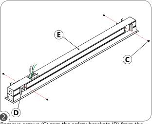
Remove screws (C) rom the safety brackets (D) from the fixture (E).
