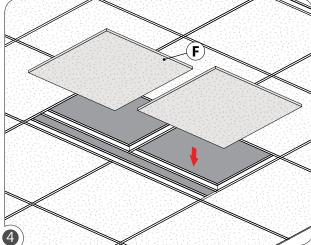
Remove ceiling tiles (F) where the fixture will be installed and adjacent tiles for easy access.
