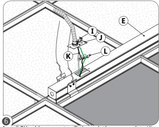
Install BX cable connector (I) through the power plate (J). Wire BX cable wires (K) to fixture (E) using the wire nuts (L). Push connected wires into fixture (E). Fasten power plate (J) to fixture (E).
