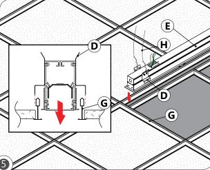
Lower the fixture (E) onto the T-bar runner (G). Ensure that the safety brackets (D) sit above the T-bars (G). For additional safety, a security wire (H) can be attached from the safety brackets (D) to the structure above.
