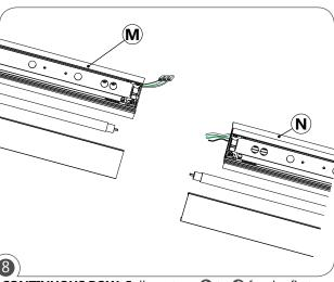
**CONTINUOUS ROW:** Follow steps **1** to **6** for the first section (M) of the fixture and follow steps 1 to 3 for the second section (N).
