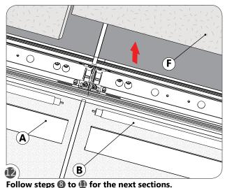
Re-install the lamps (B), optics (A) and ceilling tiles (F) at the end of the instllation process.
