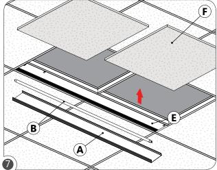
Re-install the lamps (B) and optics (A) in the fixtures (E). Ceiling tiles (F) can be placed back into their position. Power can now be turned on.
