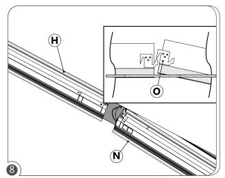
Slide fixtures (H) and (N) together and hook the brackets (O) together to join fixtures.
