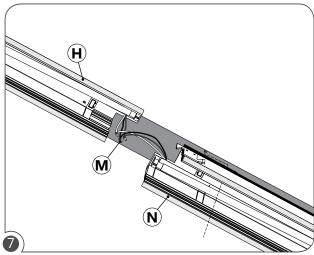
Make wire connections with quick-wire connectors (M) between the joining fixtures (H) and (N).
