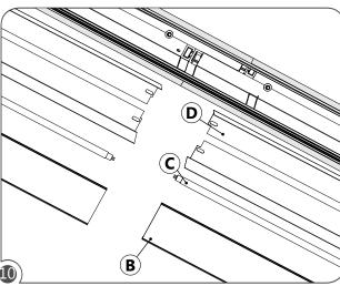
Re-install the reflectors (D), lamps (C) and optics (B).
