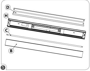
Re-install the reflector (D), lamps (C) and optics (B) in the fixtures (H). Power can now be turned on.
