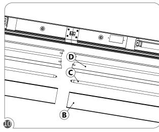
Re-install the reflectors (D), lamps (C) and optics (B).
