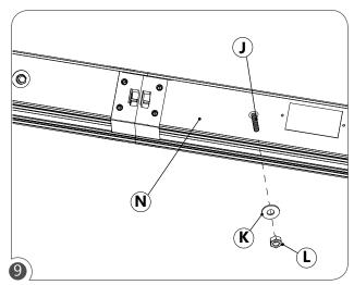
Secure fixture (N) to threaded (J) rod with washers (K) and nuts (L).
