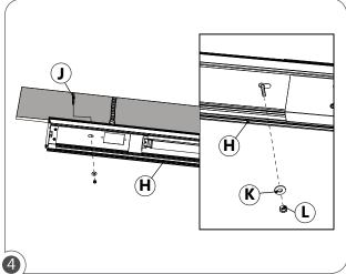
Push fixture (H) into hole in drywall, aligning 1/4-20 threaded rods (J) with holes in top of fixture (H). Secure fixture (H) with washers (K) and nuts (L).
