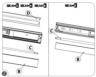
BEAM3 BEAM4 BEAM6 Remove optics (B) to gain access to lamps. Remove lamps (C) if installed. Unscrew reflector (D) to get access to the mounting holes.
