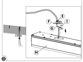
Install BX cable connector (E) through the power plate (F). Wire BX cable wires (G) to fixture (H) using the guick-wire connectors (I). Push connected wires into fixture (H). Fasten knockout plate (F) to fixture (H).
