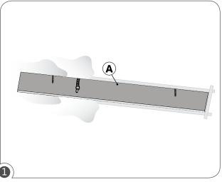
Ensure that the power to the fixture's circuit is turned off. Cut hole (A) in drywall according to the diagram and dimensions chart on the left.
