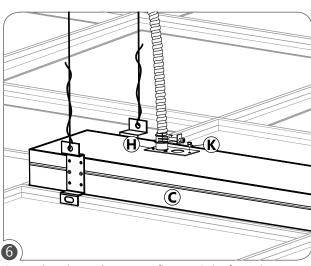
Secure knockout plate (H) to fixture (C) by fastening screws (K). Re-install the lamps and the optics.
