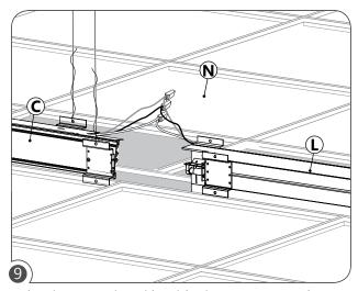
Make wire connection with quick-wire connectors (N) between the joining fixtures (C) and (L).
