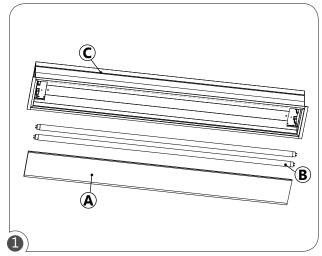
Ensure that the power to the fixture's circuit is turned off. If installed, remove optics (A) and lamps (B) from fixture
