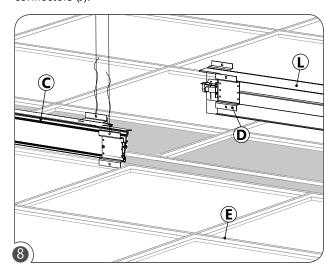
Repeat steps **1** and **2** for the second fixture (L). Raise fixture (L) above ceiling, lower fixture onto flanges of T-bars runners (E) from the top. Ensure that safety brackets (D) sit above the T-bars (E).
