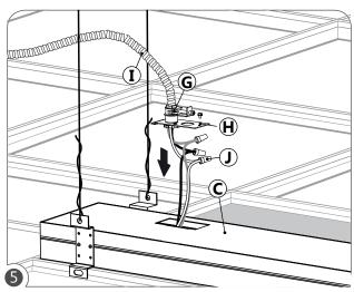
Install BX cable connector (G) in power plate (H). Wire BX cable wires (I) to fixture (C) using the guick-wire connectors (J).
