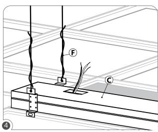
Secure support wires (F) to the fixture (C).
