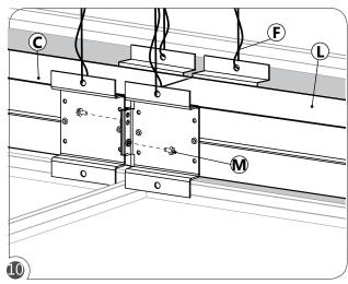
Secure the two fixtures using screws (M). Secure support wires (F) to the fixture (L). Re-install the lamps and the optics.
