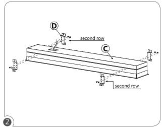
Screw safety brackets (D) to the fixture (C) using the second row of holes on the brackets.
