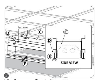
Adjust T-bar runner (E) to the fixture width. Raise fixture (C) above ceiling, lower fixture (C) onto flanges of T-bars runners (E) from the top. Ensure that safety brackets (D) sit above the T-bars (E).
