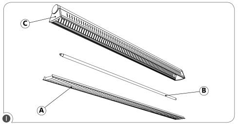
**NOTE:** Before attempting to verify and replace the ballast, ensure that the power to the fixture's circuit is turned off. Remove optics (A) by inserting your fingers inside at both ends and pull downwards. Remove the lamps (B) from the fixture (C).
