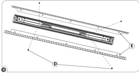
Put the reflectors (E) back in place and fasten retaining screws (D). Re-install the lamps and the optics. Power to the fixture can now be turned on.
