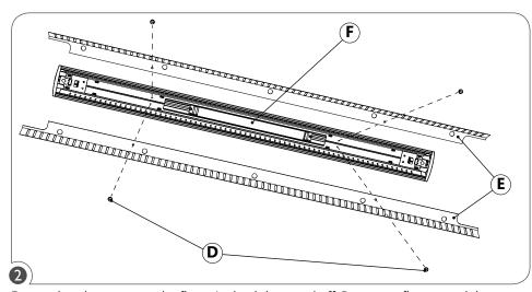
Ensure that the power to the fixture's circuit is turned off. Remove reflector retaining screws (D) to remove the reflectors (E) and reveal the ballast (F).
