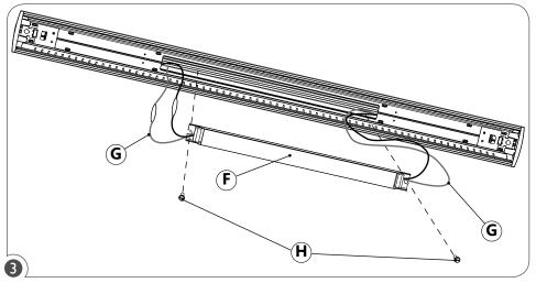
Disconnect wires (G) from the ballast (F). Remove the ballast retaining nuts (H). Replace ballast (F) and reconnect wires (G).
