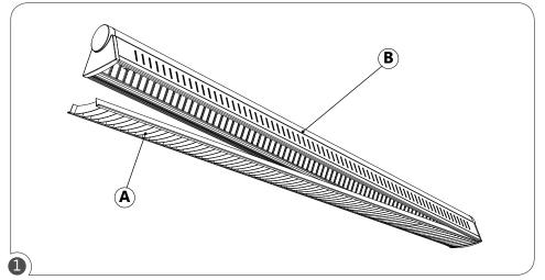
For Louver optics; Insert your fingers in the optics (A) at both ends and pull away from the fixture (B) from one end to the next end.
