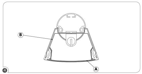
Pushing the optics (A) onto the fixture (B) from one end to the next end. The optics (A) will snap into it's final place.
