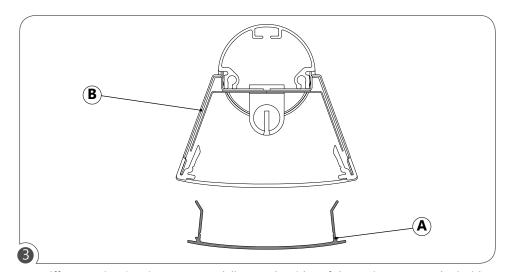
For Diffuser optics; Starting at one end, line up the sides of the optics (A) onto the inside of the fixture (B).
