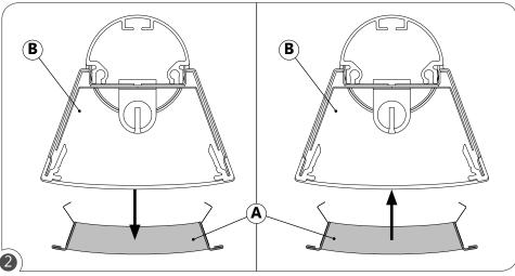
Once freed from the fixture (B), pull optics (A) downwards. To install, push optics (A) into the fixture (B). The optics (A) will snap into it's final place.
