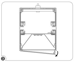
Continue removing the lens from one side of the fixture.
