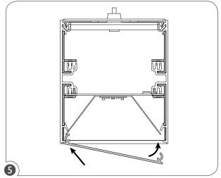
To install, slide lens inside the fixture by starting with one side and push inwards into the fixture until the lens snaps in place.
