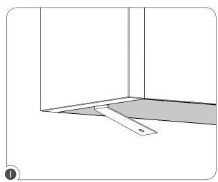
Using the provided tool. Starting at one end of the fixture, insert the bent end of the tool into the fixture lens as shown in the above illustration.
