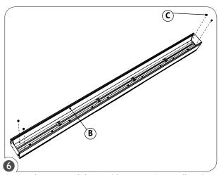
Secure the LED module (B) with screws (C). Install optics back into place.
