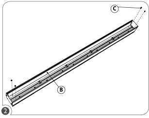
Remove screws (C) holdind the LED module (B).
