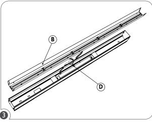
Lift the LED module (B). Disconnect the electrical wiring (D). Place LED module (B) in a safe location.
