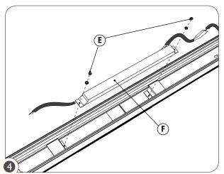
Remove the screws (E) holding the driver (F) in place. Rotate and lift the driver (F) out of the fixture. Disconnect from the fixture using the quick connectors. Connect the new driver (F) and install in place with the screws (E). FILENAME:LED.BEAM.DRIVER.INST February 19, 2014
