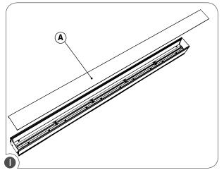
**NOTE:** Before attempting to verify and replace the driver, ensure that the power to the fixture's circuit is turned off. Remove optics (A) from the fixture.
