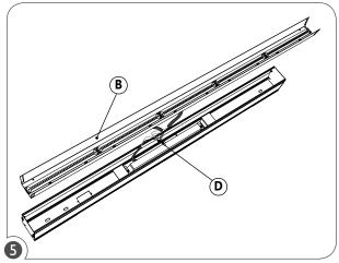
Connect the LED module (B) wires to the electrical wires (D). Install the LED module (B) inside the fixture.
