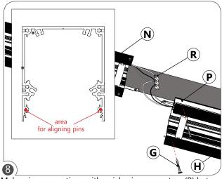
Make wire connections with quick-wire connectors (R) between the joining sections (N) and (P). Slide the second section (P) in place using the aligning pins on the section extrusion into their alocated area. Fasten the second section (P) to the drywall by drilling screws (G) through the spackle flange (H).
