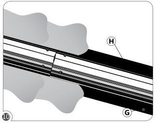
Plaster and sand over the spackle flange (H) and screws (G) of both sections to create a smooth finish.
