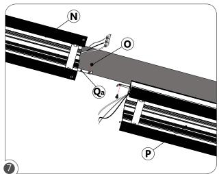
**CONTINUOUS ROW:** Follow steps **1** to **3** for the first section (N) of the fixture. Remove the screws (O) on both sections (N) and (P) joining brackets (Qa) and put away for later use.
