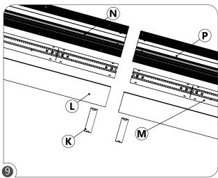
Remove the flange spacers (K) and optics (L) to gain access to LED catridges from both sections. Remove LED cartridges (M) if installed.
