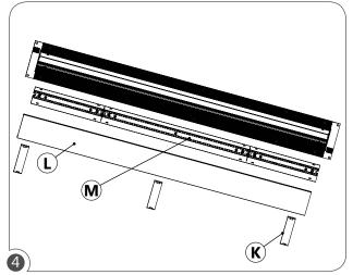
Remove the flange spacers (K) and optics (L) to gain access to LED cartridge. Remove LED cartridge (M) if installed.
