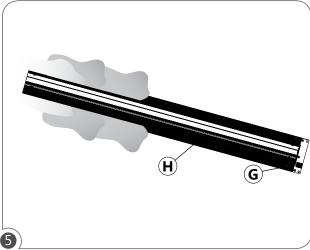
Plaster and sand over the spackle flange (H) and screws (G) to create a smooth finish.
