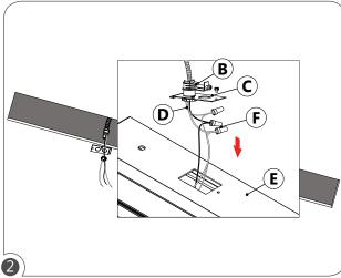
Install BX cable connector (B) through the power plate (C). Wire BX cable wires (D) to fixture (E) using the wire nuts (F). Push connected wires into fixture (E). Fasten power plate (C) to fixture (E).
