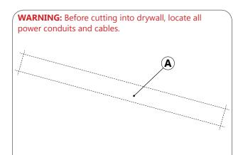
Ensure that the power to the fixture's circuit is turned off. Make an opening (A) in drywall according to the dimensions on the shop drawings.
