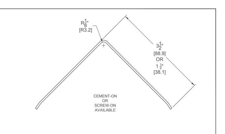
CUSTOM SIZES INCLUDE WING SIZE, HEIGHT, ANGLES, RADIUS AND GAUGE
