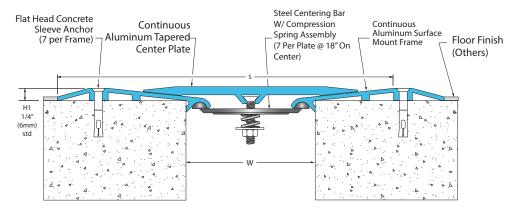
471-A02 Floor/Wall - New to Existing (4" (100mm) system shown)
