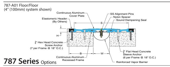
787-A01 Floor/Floor With Fire Barrier (4" (100mm) system shown)
