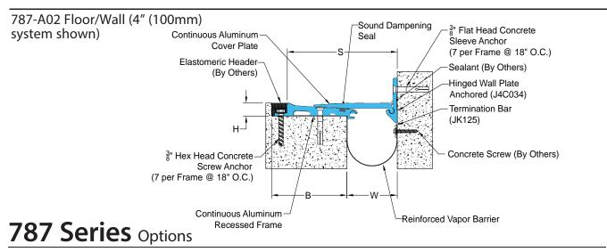
787-A02 Floor/Wall With Fire Barrier (4" (100mm) system shown)
