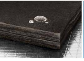
Rigid boards of resin bonded glass fibers with a reinforced foil laminate air barrier/vapor retarder. ToughGard Duct Board has a tough, durable, black mat facing applied to the air stream surface. Used to fabricate air ducts for heating, ventilating and air conditioning systems.
