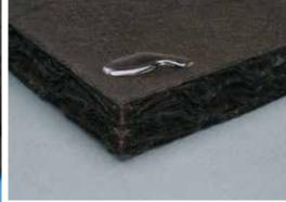
Acoustical and thermal insulation used for lining sheet metal ducts in HVAC systems. Air stream surface is overlaid with a durable black, fire-resistant composite facing. ToughGard T base mat is manufactured with textile and rotary fibers bonded with a thermosetting resin system.
