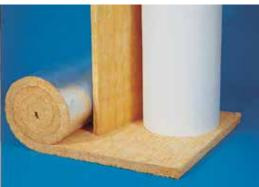
Flexible blanket of selectively oriented glass fibers firmly bonded together with a thermosetting resin. Available with either Foil Scrim (FS) or ASJ (All Service Jacket) vapor retarder facings. Used to control heat loss or gain in large diameter piping, tanks and equipment.
