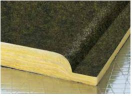
Ultra\*Duct Black Duct Board is a rigid board designed for fabrication into supply and return air HVAC ductwork. Composed of resin bonded glass fibers with a reinforced foil laminate air barrier/vapor retarder facing applied to the outside surface, and a fiber glass textile mat bonded to the air stream surface.
