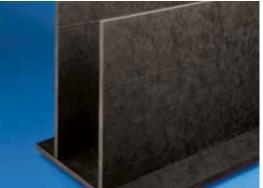
Semi-rigid acoustical and thermal insulation board composed of glass fibers firmly bonded with a thermosetting resin. Air stream surface is overlaid with a tough, durable, fire-resistant black composite surface. Used for lining large sheet metal HVAC ducts and plenums.
