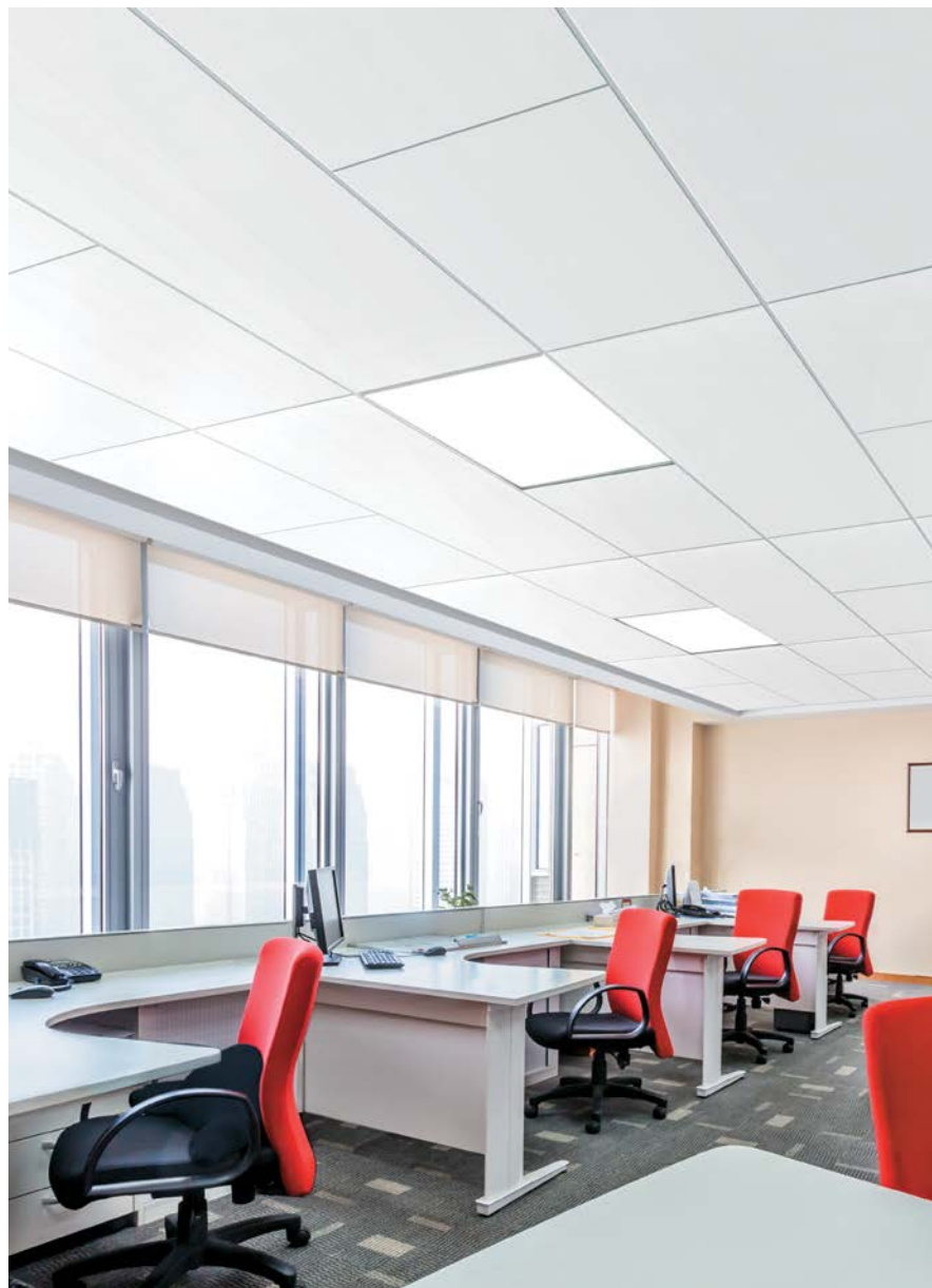
Lyra® PB Square Tegal panels with Suprafine® 9/16 suspension system
