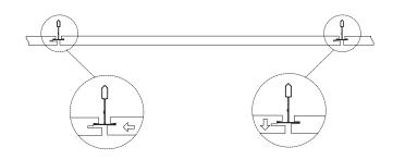
**STEP 3:** Slide the panel so that the registration kerf on edge "B" engages the grid flange. Ensure that the access kerf on edge "A" drops down into the correct position.
