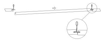
**STEP 2:** Raise the "B" edge of the panel, the registration kerf, into the grid opening until the kerf lines up with the grid flange.
