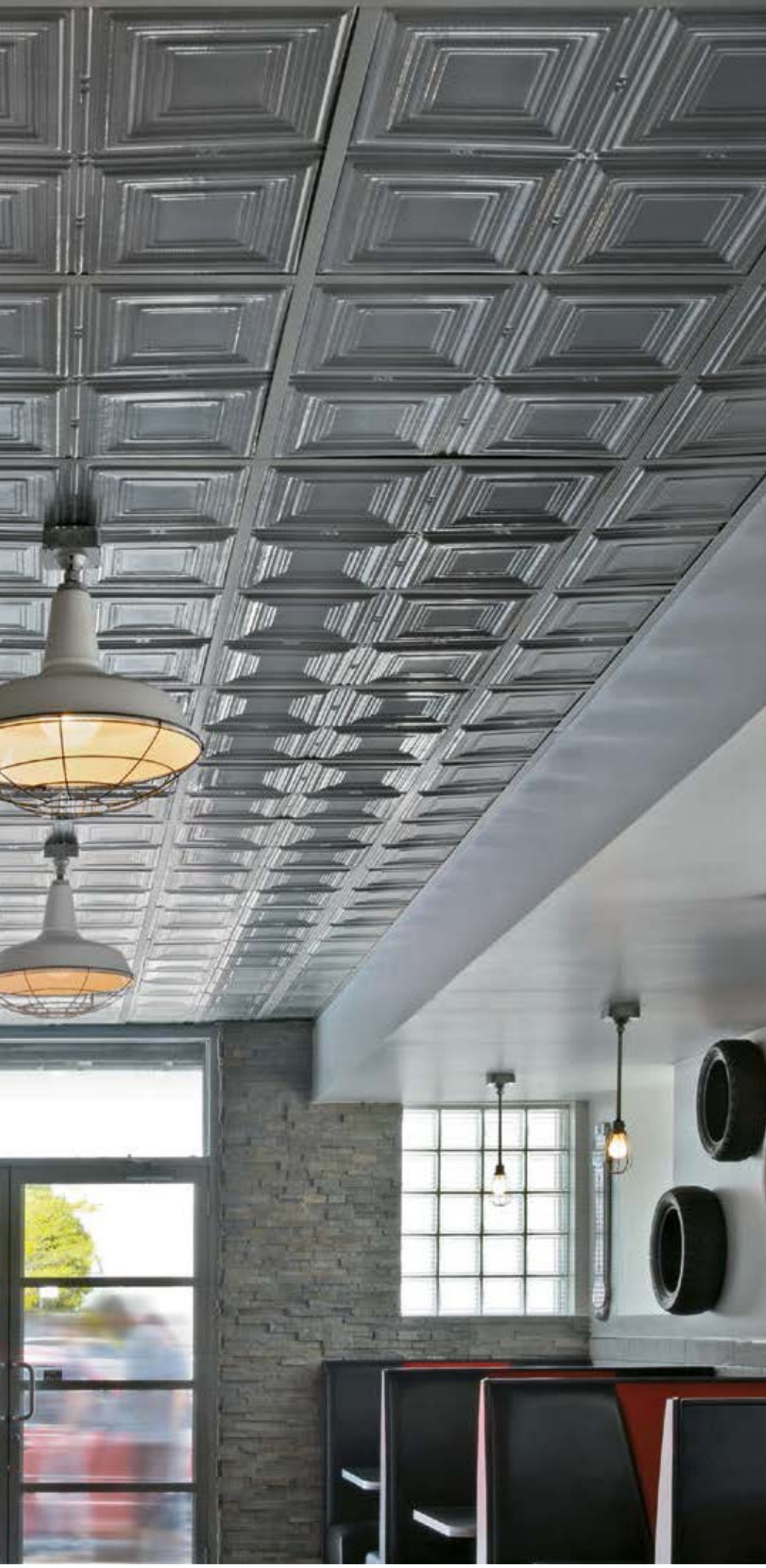
MetalWorks™ Tin 15/16" Tegular item 56007 Extra Microperforated in Lacquered Steel; The Burger Garage, Long Island City, NY
