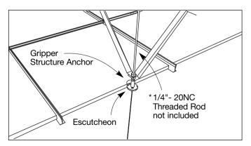
Use the optional escutcheon kit accessory to conceal the structure gripper anchor when installed above the ceiling level.
