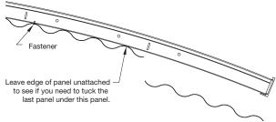
**11.6** For the last panel, again make sure the finished edge lines up line below.
