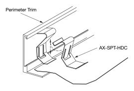
StrongBack™ Support Channel is a steel component that carries the weight of the outer 2' of most installations. Use of the StrongBack allows the hangers to be placed 2' from the edges on installations 6' wide or greater.
