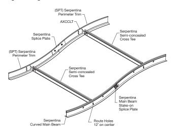
Serpentina Perimeter Trim Clips (AXCCLT clips) are used for the attachment of the suspension system (main beams and concealed tees) to the Serpentina perimeter trim. Hold the insertion tab with pliers and twist to lock into place.
