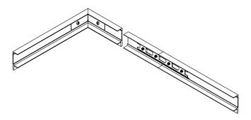
**8.2 DO NOT OVERTIGHTEN SETSCREWS.** Excessive torque will result in deformation of the trim that will show on the finished surface.
