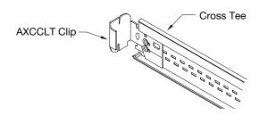
**6.3** Install STAC clips (as shown below) onto the cross tees that intersect with the two main beams located in the center of the Formations cloud. (These main beams create the 4" opening for the lighting fixture). The STAC clips hold the cross tees in their correct position.
