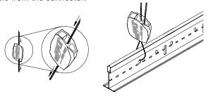
**5.2** Attach Axiom Clips (item AXCCLT) to each end of the main beams by positioning as shown in the drawing. The top of the clip should touch the bottom of the bulb of the suspension system and the end of the main beam should contact the thumbnail stop on the clip. Secure each clip with two poprivets or #8 sheet metal screws (note that pop-rivets are preferred over screws because they will not interfere with the placement of the ceiling panels).
