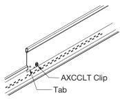
**7.3** Cut away the end detail on the cross tees that will engage the Axiom® trim. Attach an Axiom Cross Tee Clip to the end of each cross tee as shown.
