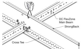
**7.2** Bend the tabs at the ends of the StrongBack™ Support Channel as shown so that they will fit under the bottom of the bulb of the cross tees and secure with a #8 x 9/16" screw.
