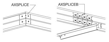
**8.5** DO NOT OVERTIGHTEN SETSCREWS. Excessive torque will result in deformation of the trim that will show on the finished surface.
