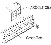
**7.4** Note that pop-rivets are preferred over screws. Align the clip such that the lower two holes in the three-hole line match up with the holes in the end of the cross tee. Insert two fasteners through the cross tee and into the clip.
