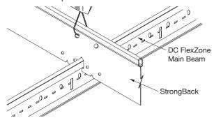
**6.2** Attach Axiom Cross Tee Clips (item AXCCLT) to each end of each main beam by positioning as shown in the drawing. The top of the clip should touch the bottom of the bulb of the suspension system and the end of the main beam should contact the thumbnail stop on the clip. Secure each clip with two pop-rivets or #8 sheet metal screws (note that pop-rivets are preferred over screws because they will not interfere with the placement of the ceiling panels).
