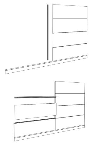
Vertical splines can be secured to the wall using appropriate fasteners. The vertical splines capture the vertical edges of the panels. The horizontal and vertical splines must meet at a 90-degree angle.
