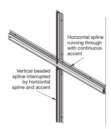
The installation of the ground strip, baseboard and finish molding is done the same as with vertically mounted panels. Remember to cut horizontal accent trims that protrude from the face of the panels 3/8" short of the end of horizontal panels. This will accommodate the fit of the finish molding installed vertically at the end of the installation.
