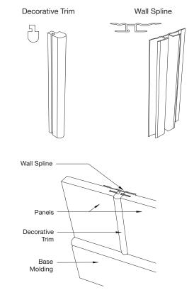
If the trim does not protrude from the face of the panel, cut the trim so it rests on the ground strip at the bottom and extends to the top of the panel.
