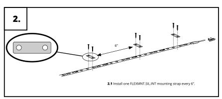
Installation Directly to Mounting Surface
