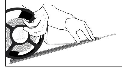
Installation with Recessed Channel: No Spring Clips
