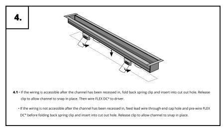
Installation with Recessed Channel: With Spring Clips
