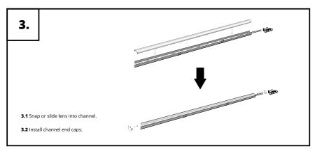
Installation with Surface Mounted Channel
