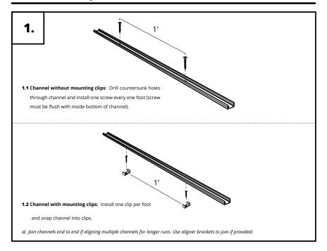
Installation with Surface Mounted Channel
