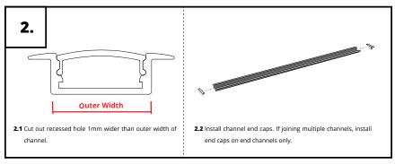
Installation with Recessed Channel: No Spring Clips
