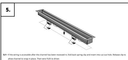
• If the wiring is not accessible after the channel has been recessed in, feed lead wire through end cap hole and pre-wire FLEX, then fold back spring clip and insert into cut out hole. Release clip to allow channel to snap in place.
