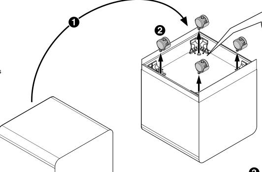
TIP: Tapping bottom metal panel with a hammer may help with pulling caster loose, or pry with crowbar under metal lip of caster to remove pintle.
