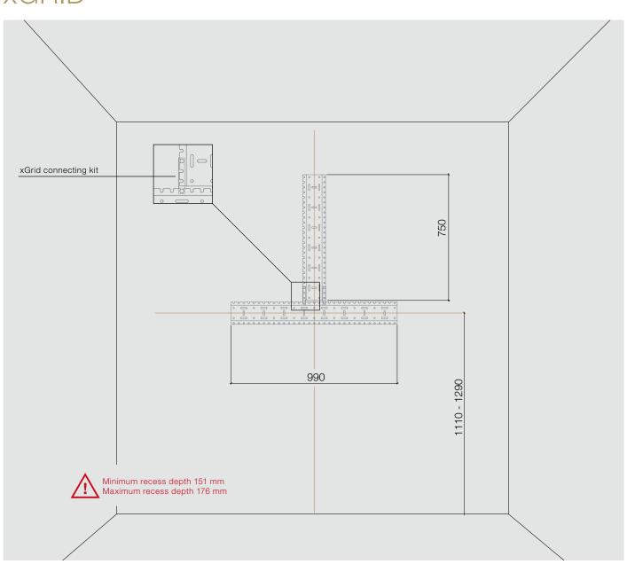
Three different lengths of xGRID installation track are available: 990/750/510 mm.
