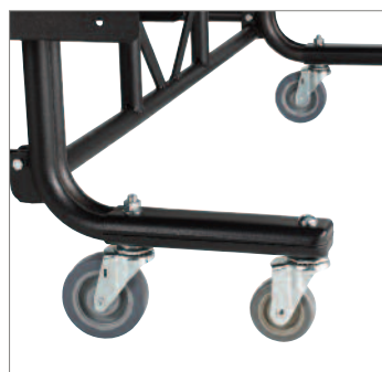
C Outrigger casters enable the table to fold flat and nest, minimizing table storage footprint while still exceeding UL tip-over requirements.
