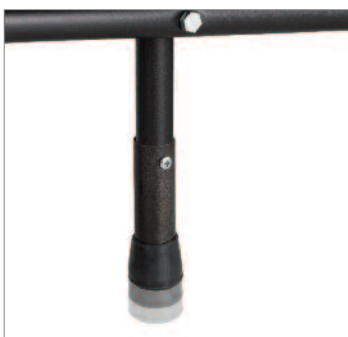
B Self-adjusting support legs are spring loaded to ensure contact with uneven floors and to keep the table from rolling away while the table is in the down position.
