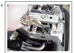
Using a pliers remove the black locking pin of the broken handle by pulling away from mechanism. Place locking pin aside.
