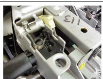
Ensure locking pin is "snapped" into postion. Note: The pin is in position when it is the same depth as pin on opposite side.
