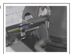
Position right lateral cover under opposite side of lower mechanism shroud and under height adjustment, back adjustment stems.
