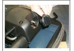
Pull on the tension knob to remove it from the front of the mechanism.
