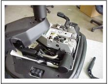
Rotate the bottom mechanism shroud towards the back of the chair to expose the mechanism as shown above.
