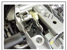
Slide the Locking Pin back into position, the first hole for the forward seat tilt rod and the second hole for the back lock. Place the wire inside of the locking pin loop.
