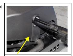
Position left lateral shroud under activation stem and into cover shroud.
