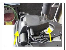
Remove the bottom mechanism shroud pictured above by pulling on the bottom of the shroud where indicated.
