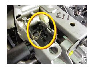
Place the wire inside of the locking pin loop
