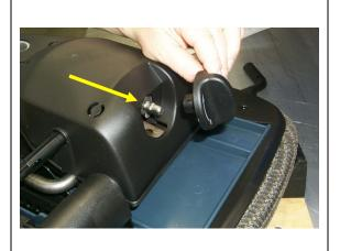
Remove tension knob from front of mechanism. PC.06.4011.BL
