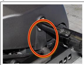
Position left lateral shroud under activation stem and into cover shroud. PC.06.4012.L.BL
