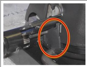
Position right lateral cover under opposite side of lower mechanism shroud and under height adjustment, back adjustment stems PC.06.4012.L.BL
