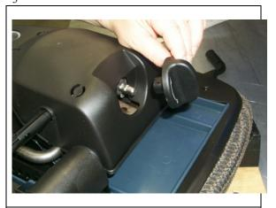
Replace tension knob onto front of mechanism
