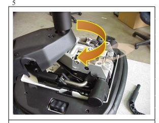
Lift & rotate the mechanism shroud towards the back of the chair to expose the mechanism as shown above.
