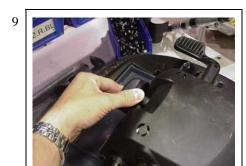
Remove tension knob from mechanism by pulling directly away from mechanism.
