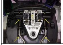
Using a #3 phillips screwdriver, remove the four bolts that attach mechanism to seat board.
