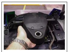
Remove lower mechanism shroud by lifting shroud
