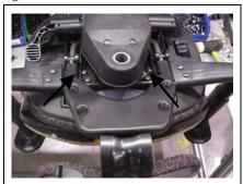
If chair has arms: Remove the four bolts indicated above that attached the arms to mechanism and place parts aside.
