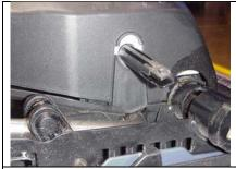
Position LH lateral cover, removed in step 11, under forward tilt rod.
