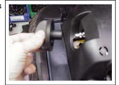
Attach tension knob, removed in step 9, to mechanism. Knob is a press fit onto mechanism.
