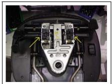
Remove right and left lateral covers from under handles. Cover position is shown above.
