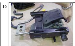
Get new mechanism, PC.15.4001, and attach upper mechanism shroud removed in step 15.
