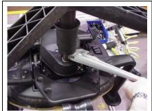
Using a pipe wrench or vise grip, place it on cylinder as above and twist to free cylinder. Remove base assembly and place aside.
