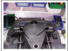
Remove right and left spring caps shown above by removing...
