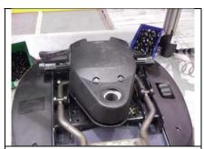
Loosely set lower mechanism shroud, removed in step 10, on top of mechanism as shown.
