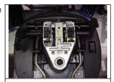
Using a flat screwdriver and hammer, remove the height adjustment handle from the mechanism, place aside.
