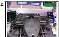
Snap the two spring covers, removed in step 7, onto mechanism.
