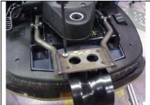
Using a #3 phillips screwdriver, remove the four bolts that attach the j-bar to the mechanism. Hold back so it does not fall when removed.
