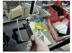
7. Locate the spring side bushing (PC.06.2562.BL) and slide it onto the ganger. Slide the spring (PC.45.5510) over the end of the ganger.
