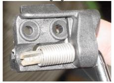
3. Rotate the ganger one full turn while holding the bushing with the spring stationary, making the ganger spring loaded. Snap the bushing into place.
