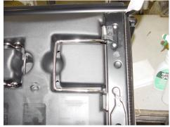
9. Locate the non-spring side bushing (PC.06.2564.BL). Snap the bushing into place.
