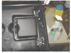
10. Locate screws (PC.12.0583). Secure the bushings with the screws to hold the ganger in place.
