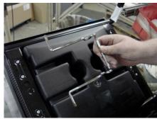
2. Locate the spring side bushing (PC.06.2562.BL) and slide it onto the left ganger. Then, slide the spring (PC.45.5510) over the end of the ganger.
