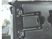
6. Locate the parts for the right side ganger assembly. Locate the right side ganger (male 87.7831)
